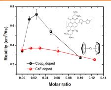
Performance and air stability is highly improved in n-type organic field-effect transistors by solution-based chemical doping. The doping effects are systematically investigated the relationship between doping concentration and electrical characteristics as well as the evolution in polymer crystallinity revealed by synchrotron X-ray diffractions.
