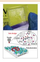
Surface charge reversal method for highresolution inkjet printing of functional water-based inks is revealed. The proposed approach modifies the surface energy of hydrophobic substrates by coating with a polyelectrolyte layer in order to overcome dewetting effects as well as to improve adhesion and printing resolution. A suitable metal complex ink is formulated, which can be processed via inkjet printing.
