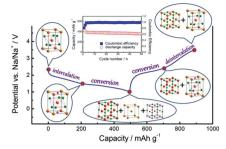
A high-capacity cathode for a sodium battery is presented. FeO $_{0.7}$ F $_{1.3}$ /C nanocomposite exhibits a high initial discharge capacity of 496 mAh g $^{-1}$  in a sodium cell at 50 °C. A reversible capacity of 360 mAh g $^{-1}$  is retained at the 50<sup>th</sup> cycle, demonstrating superior cycleability. Both intercalation and conversion reactions are revealed during the discharge—charge process of the FeO $_{0.7}$ F $_{1.3}$ /C - Na cell.
